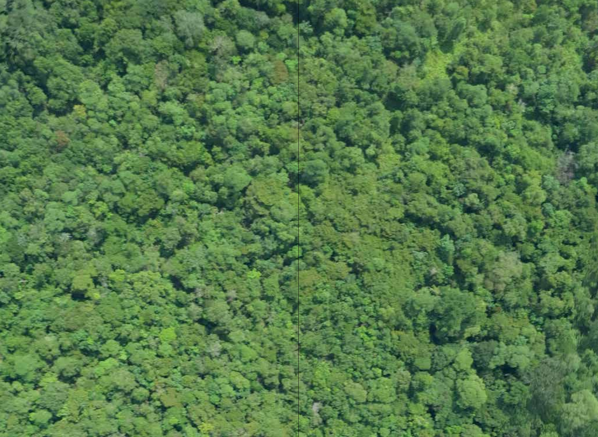
Fig. 06. Drone imagery is fundamentally composite; photogrammetry processing involves the identification of common pixels across multiple images, which can then be programmatically synthesized into a single, high-resolution image, as in this drone photograph of the forest canopy in Central Kalimantan.
